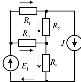
$$R_{EQ1} = R_4 + \frac{R_3(R_1 + R_2)}{R_3 + R_1 + R_2} = 29,52 \Omega$$
