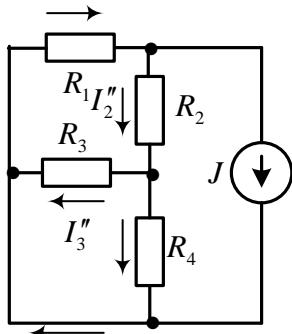
$$R_{234} = R_2 + \frac{R_3 R_4}{R_3 + R_4} = 23,33 \Omega$$
